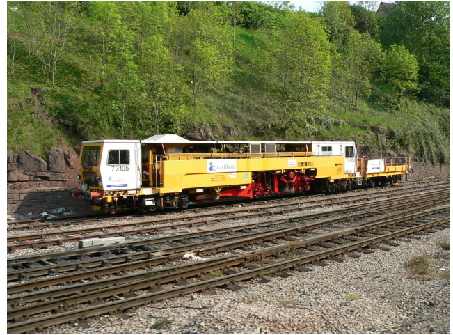
Fig. 4. Plasser & Theurer 09-16 CSM Tamper / Liner[12].
