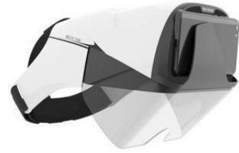
Fig. 1. Optical see-through head-mounted display. The smartphone slot can be seen at the front of the HMD.
